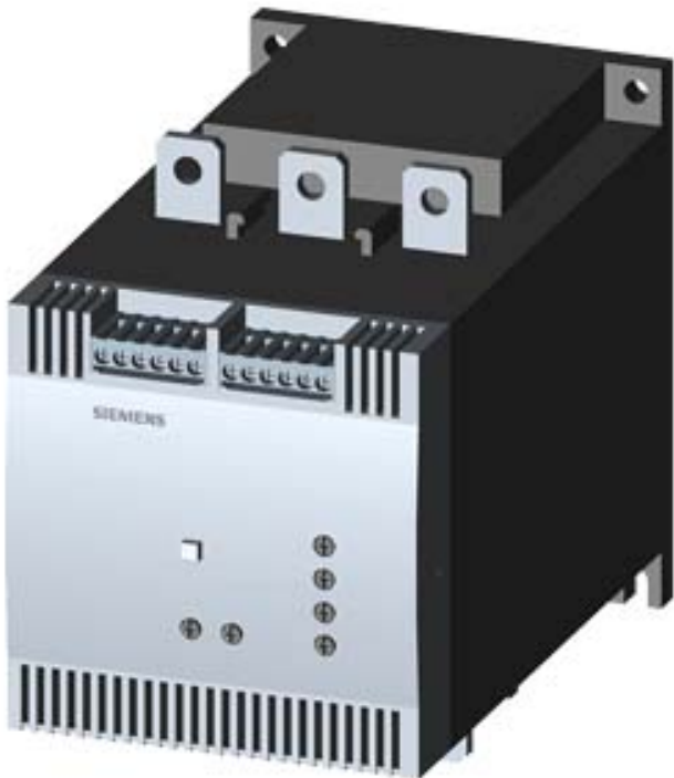
SIRIUS SOFT STARTER, S12, 205 A, 200 HP/575 V, 50 DEG., 400-600 V AC, 115 V AC, SCREW TERMINALS
