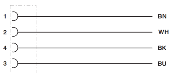
Contact assignment M12-plug and M12-jack
