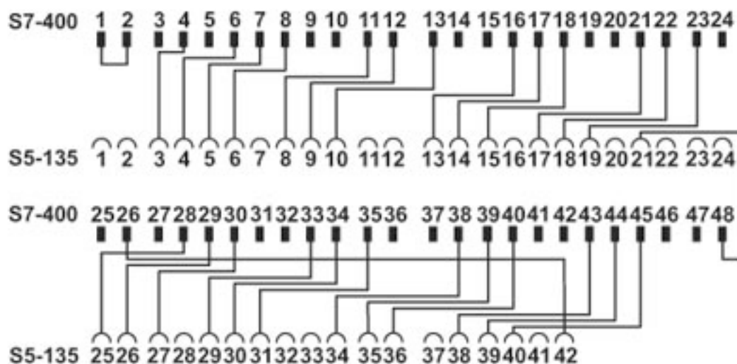
Connection scheme FLKM S135-470-4UC/U/S400
